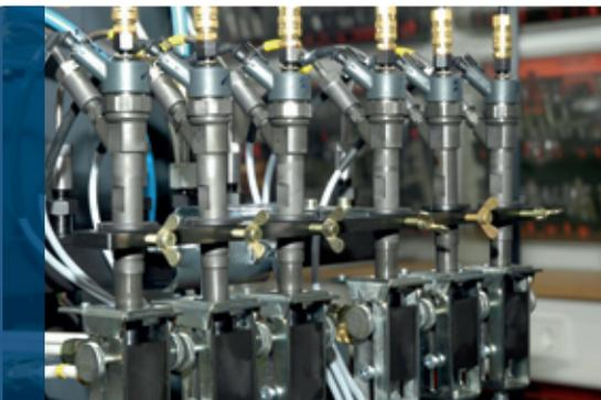
mounting plate. At the core of repair stage 3, however, is a special type of software that provides diesel mechanics with the organisational set-up of all the tools and adapters to be used and with all the necessary set-points. The full set makes it possible to work on injectors with the same degree of precision as in the factory.
