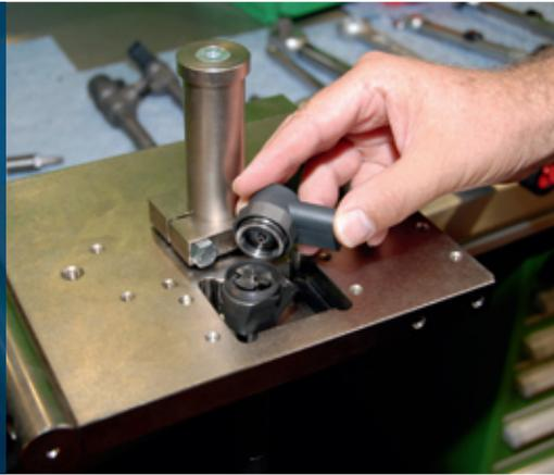
nozzle-retaining nut to the injector is one of the determining factors in making the repair a success. Even the tiniest inaccuracies can result in leaks between the injector components. To this end, Bosch's customer service and research engineers worked together to develop a special screw-fitting process specifically for workshop applications, which, if precisely adhered to, yields the same stability as that of screw-fitting processes used for mass production on costly machinery.
