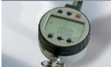
Digital dial gauge for tolerances of 1 µm
