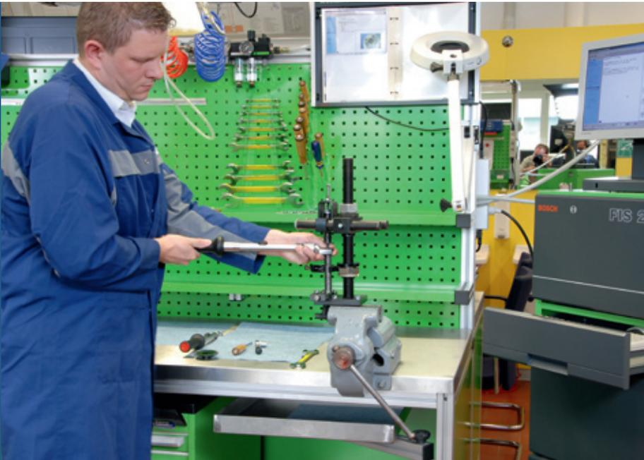
The repair of Common Rail injectors requires maximum cleanliness. Repair stage 1 only involves replacement of the nozzle. Photo: Linzing
